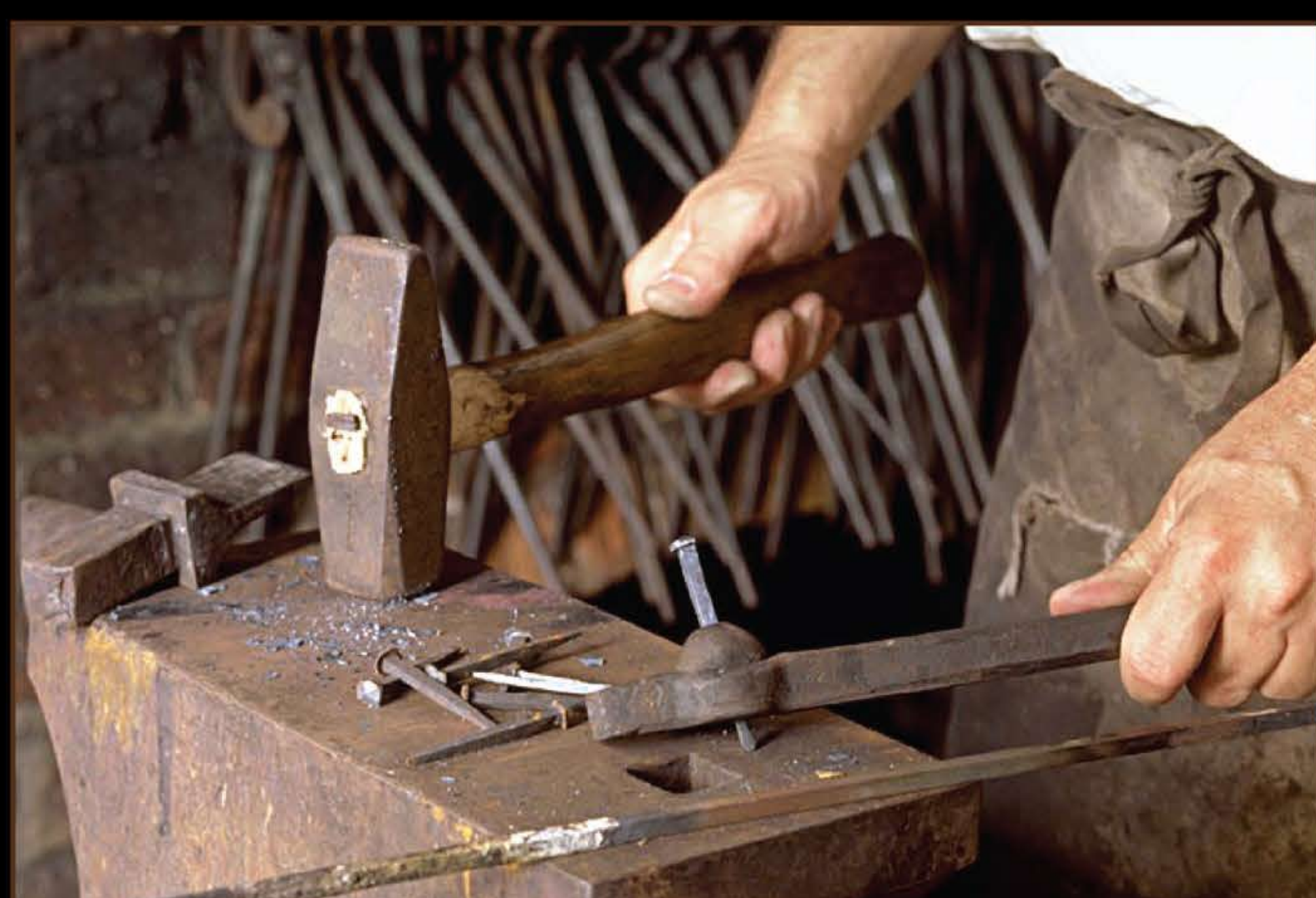
▲ Nails made by a blacksmith are four sided and taper toward the tip.
