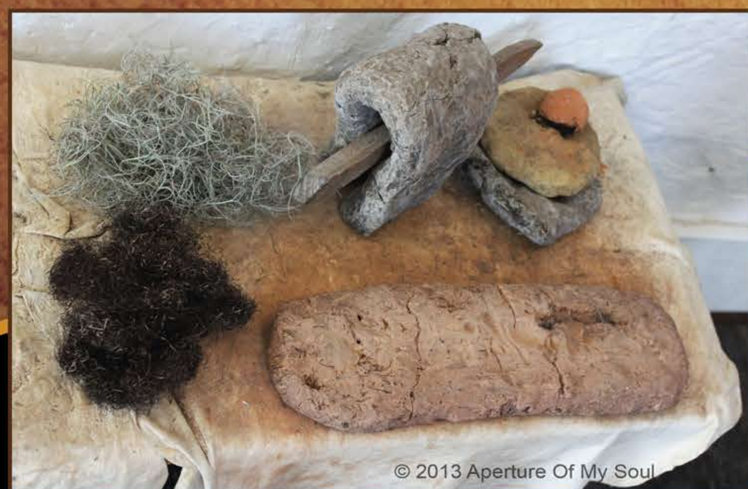
Bousillage found at Fort St. Joseph (image on left) was made with clay and straw (image on right) ▲
