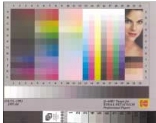
Figure 5. Image printed with zero dot gain correction curves, adjusted black point level, gray balance correction curves and custom ink settings.
