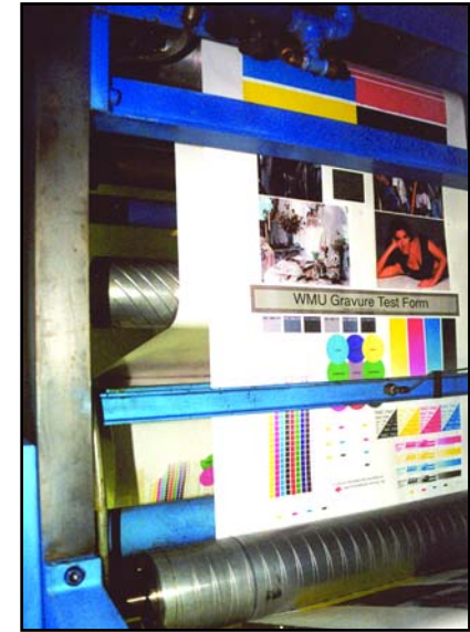
Four-color form on gravure printing press.
