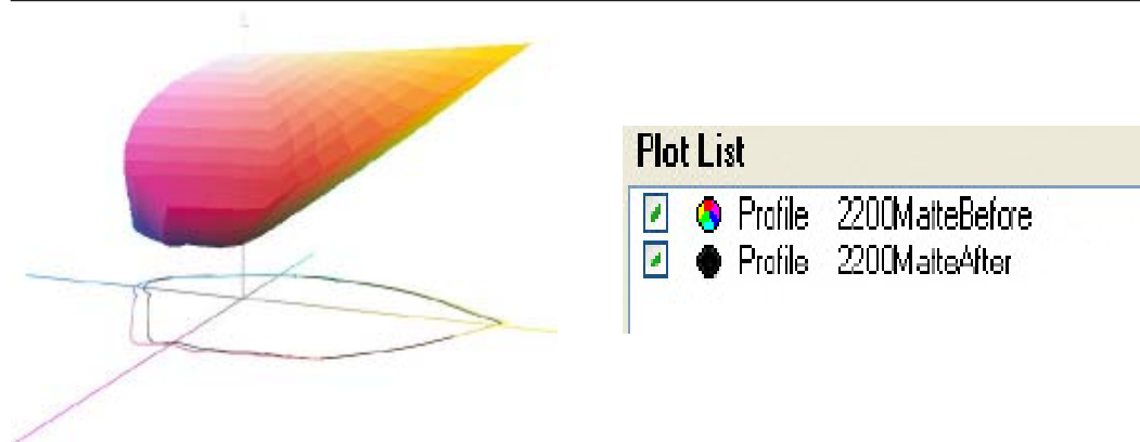
Fig. 6. Comparisons of color gamuts before and after fading test for Epson 2200 and Archival Matte substrate.
