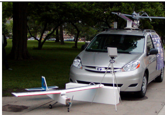
Flying Machines: Dr Kapseong Ro led the development of a plane with solar panel wings (in front of the van) and teamed up with Dr. Jun-Seok Oh and a team to develop the unmanned aerial vehicle (UAV) for traffic and emergency surveillance that is on top of the van. Team members DaeWoon Park and Taeseung Kuk also participated.
