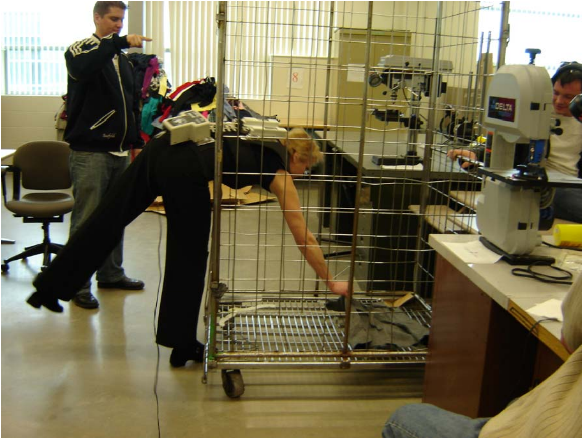
Ergonomics Testing for Ease of Reaching Items in the Redesigned Transit Cart
